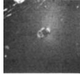
Fig. 4. The inclusions in \alpha -Si:H detecting by NLC. Magneron sputtering, magnification 300\times , MBBA, t^\circ=18^\circ\text{C}
